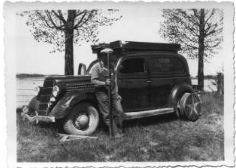
Raymond D. Fisher with a truck that read HESS Radio - Electric Zurich. Look at the take up reel attached to the back tire. The 35 to 36 Ford Sedan Delivery was put up on a jack and the vehicle put into drive to spin the reel. This was done to reclaim the steel wire to be reused at another location. Innovative technology for the time.
